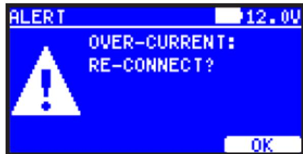
**WARNING:** *you run the risk of damaging your battery, and powered devices if you continue to try and draw power from the battery.*
