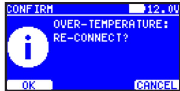
**WARNING:** *you run the risk of damaging the Battery Monitor if you override the shut off.*
