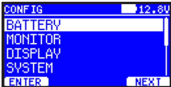
Press the **NEXT** button to scroll down to highlight the desired item, then press the **ENTER** button to select.
