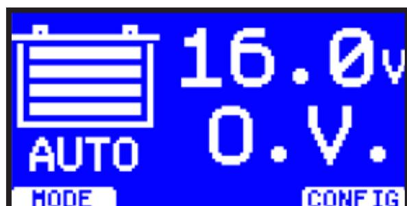
The Battery Monitor will automatically restore power to the output load when the voltage returns below a factory pre-configured setting: Lead Acid = 14.2V, AGM = 14.6V, Calcium 15.3V.
